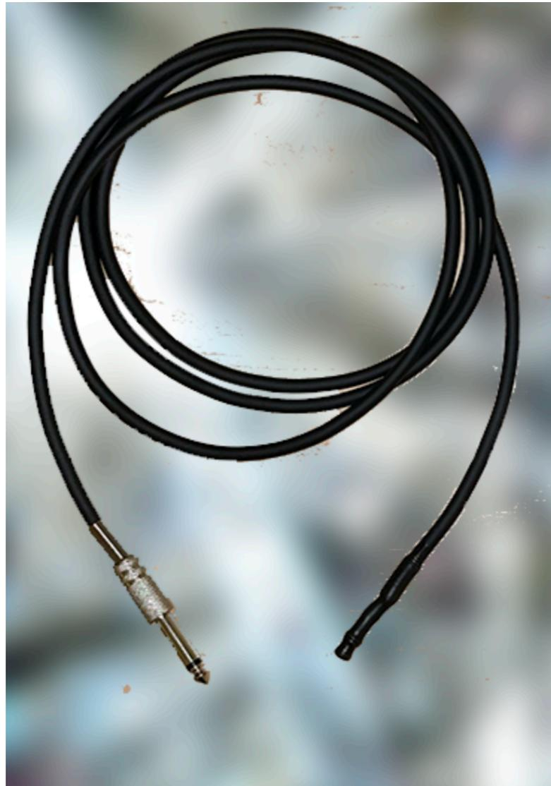
My EMF microphones (electromagnetic field microphones) are designed to detect electromagnetic fields rather than acoustic vibrations, translating invisible EM activity into audible signals. Each microphone consists of a tightly wound copper coil (either air-cored or wrapped around a small ferromagnetic core) soldered directly to a shielded microphone cable and terminated at a 1/4-inch jack.
