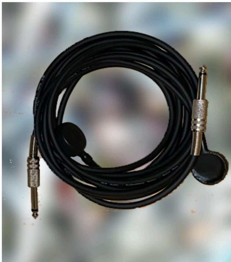
My custom hydrophones are built from waterproofed piezoelectric disk transducers designed to capture pressure waves in underwater environments. Each piezo element is housed inside a custom 3D-printed enclosure which is subsequently filled with a casting resin formulated to match the density of water. Utilizing resin of this specific density ensures that the hydrophone accurately reproduces underwater sound with reduced spectral deviation, distortion, or muffling.
