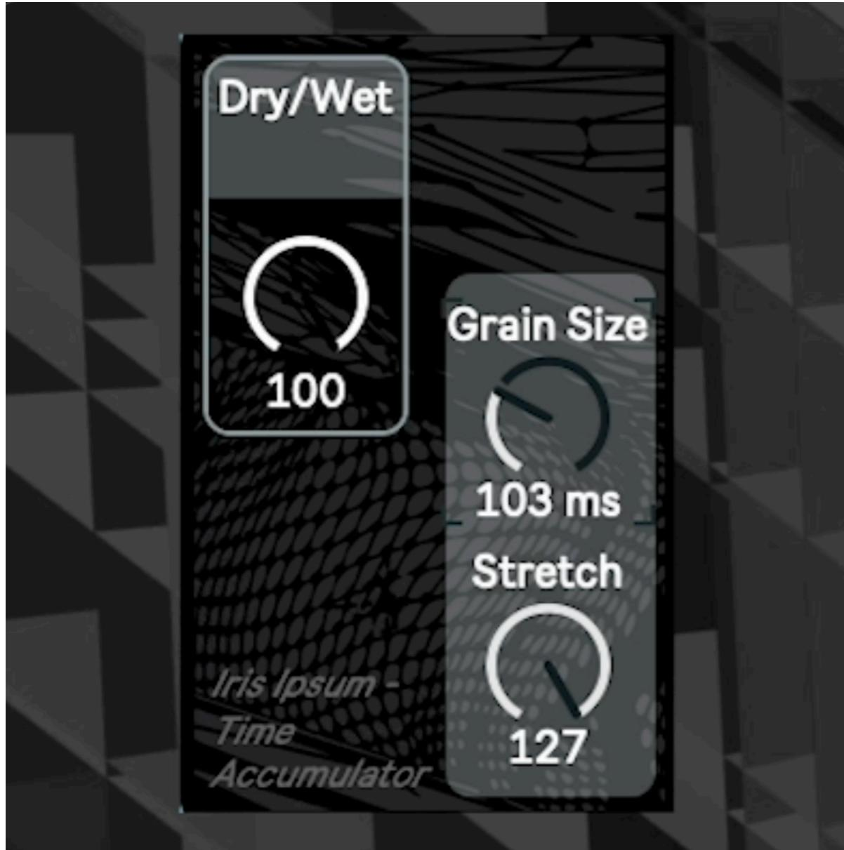
Time Accumulator is a real-time temporal processing device that generates stretched, frozen, and smeared audio textures by scanning through a continuously updated circular delay buffer. Rather than employing granular or frequency-domain techniques, the device performs its time manipulation entirely in the time domain by dynamically adjusting the read position of a long delay line.
