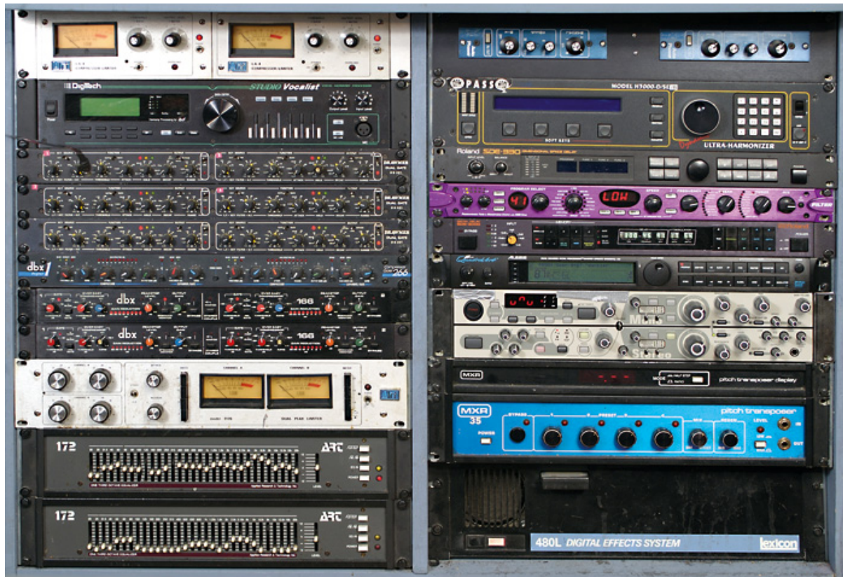
Figure 8. Two full racks of recording studio rack-mounted effects processors
