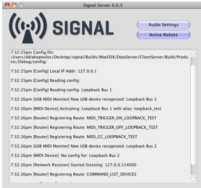
FIGURE 3.2: The Signal/Server logging window
